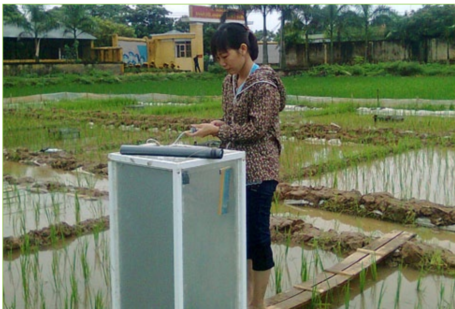
Chamber method for sampling and measuring methane and nitrous oxide emissions (photo from IAE 2016).
