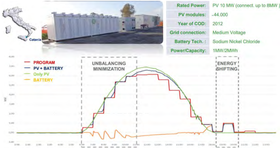
Figure 3.5: Solar Photovoltaic Installation with a Storage System
