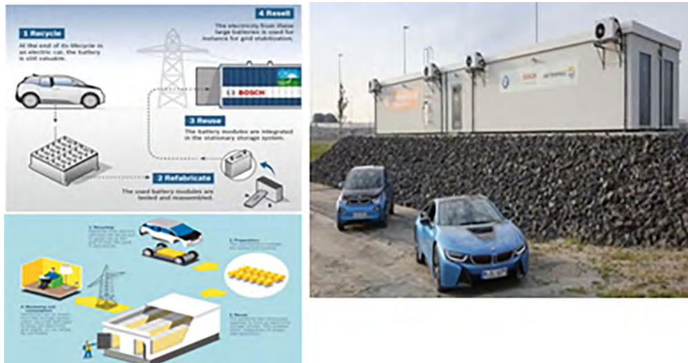
Figure 4.6: BMW–Bosch Second-Life Electric Vehicle Battery Demonstration Project
