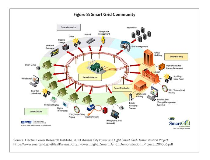
84. A smart meter is something that is often heard when discussing smart grids. A smart meter is a device that enables two-way data transfer between the customer and the distributor; data examples are electricity consumption, electricity production, tariff options (time of use), and grid health.
