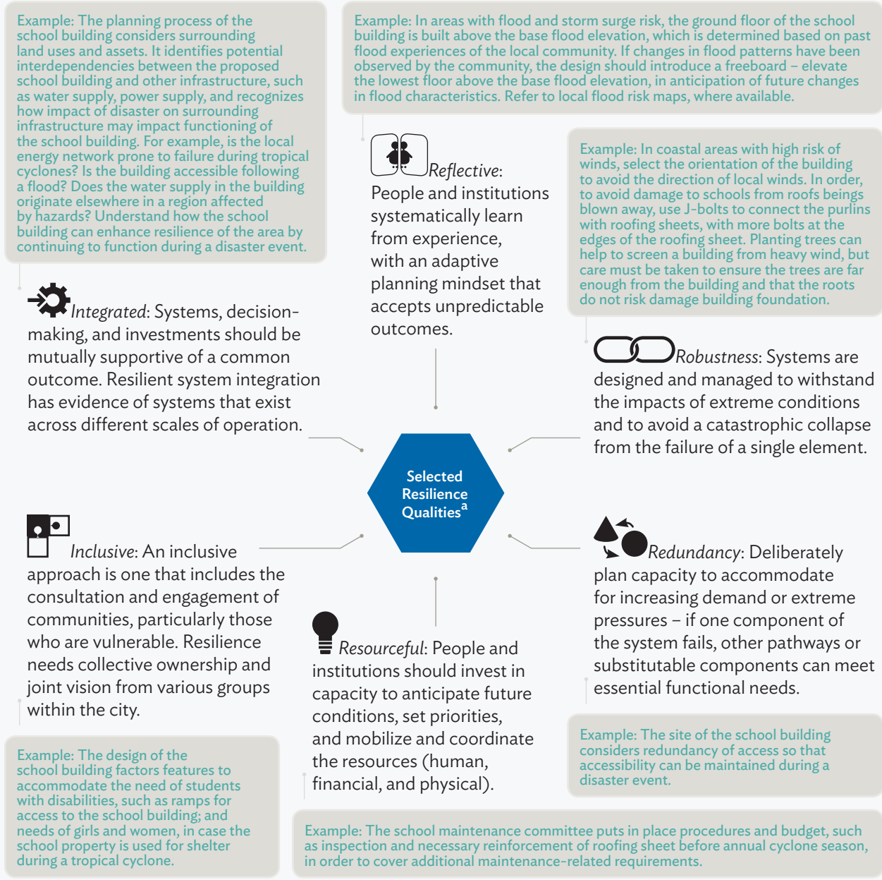
Figure 3: Integrating Resilience Qualities in the Design of School Buildings Located in Typhoon-Prone Areas
