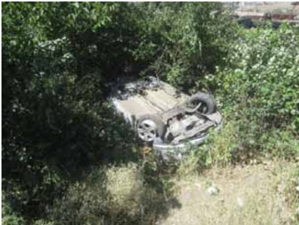
A critical side slope (steeper than 1V:3H) increases the risk of rollover crashes. In turn, this increases the risk of serious injury or death for vehicles' occupants.
