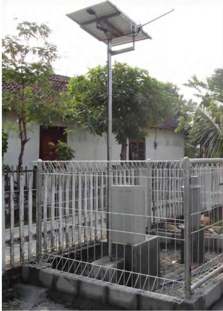
Automated rain-gauge station at Pajeng. Automated rain gauge sends alert to community members when rainfall exceeds the threshold (photo by the Asian Development Bank).
